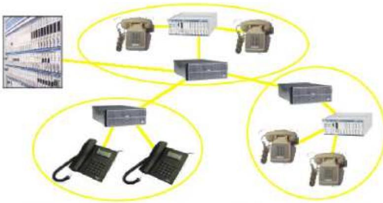
One of iPBX most powerful features is its ability to link remote offices of a SME (Small to Medium Enterprise) together. The above diagram shows how you can build individual small PBXs for multiple offices using iPBX, and then link them together transparently into a single network.
